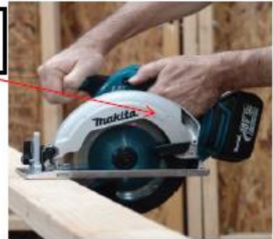
Self-adjusting blade guard
